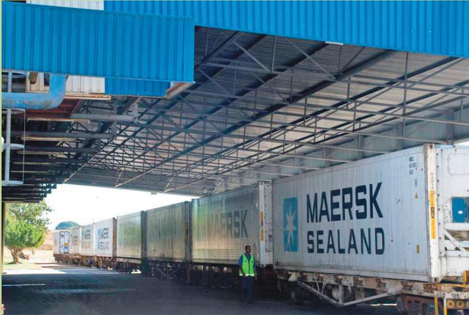
*The reefer containers were connected to a power supply at Cold Harvest while the train was being loaded, so as to maintain the cold chain. The Cold Harvest facility at Paarl ( part of SAFT) packs and cools fruit and has a storage capacity for 6400 pallets*
